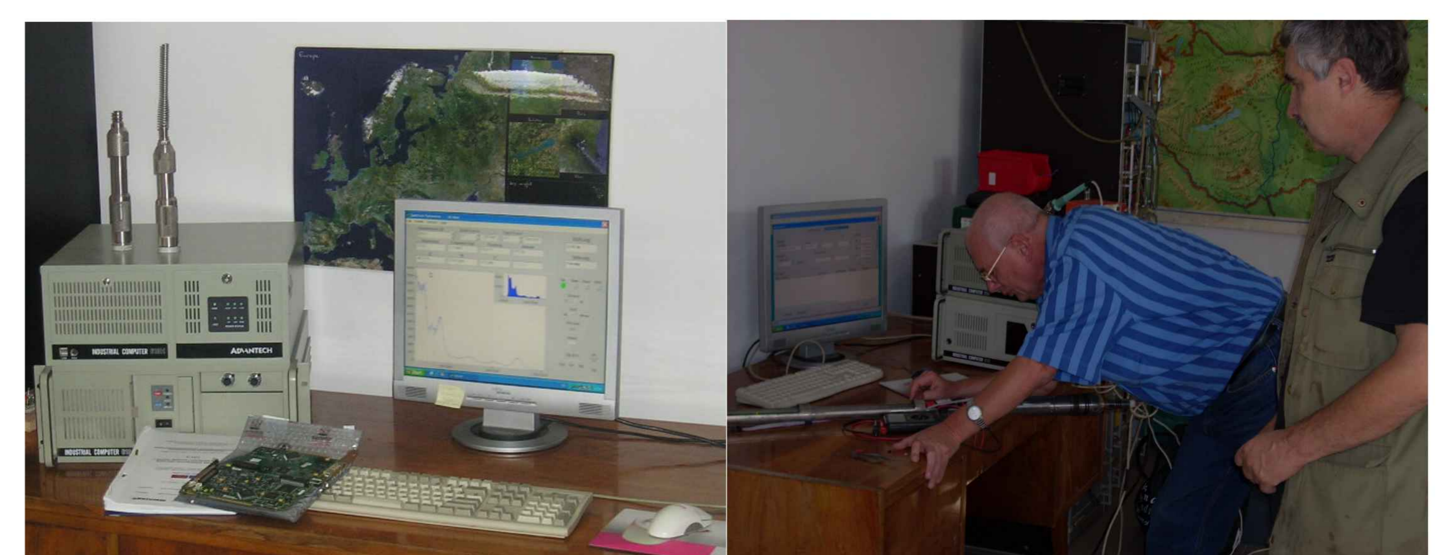
Surface measuring unit built in an industrial computer case and testing the measuring probe
